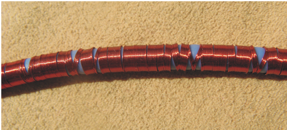
Figure 3. Coil former bulging out between the windings
